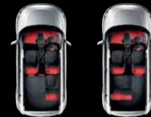
60:40 seat folding / seat variation: Soul will never cramp your lifestyle. The rear seats split 60:40 and the backrest folds down almost flat to create 570 litres of space – enough for two mountain bikes.
